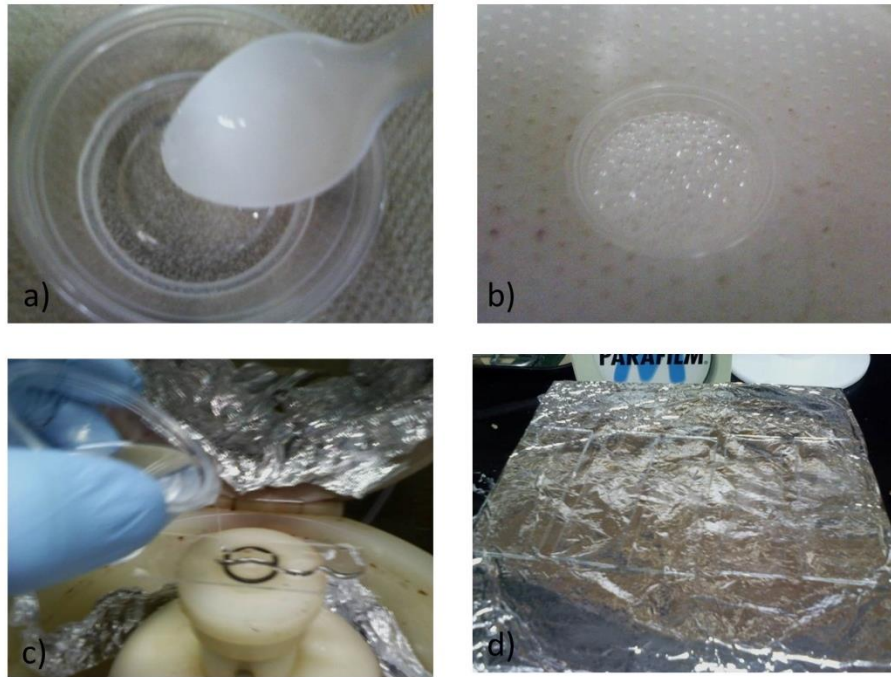
Figure 3: Stages of PDMS slide preparation a) mixing, b) degassing, c) spincoating, and d) baking.
