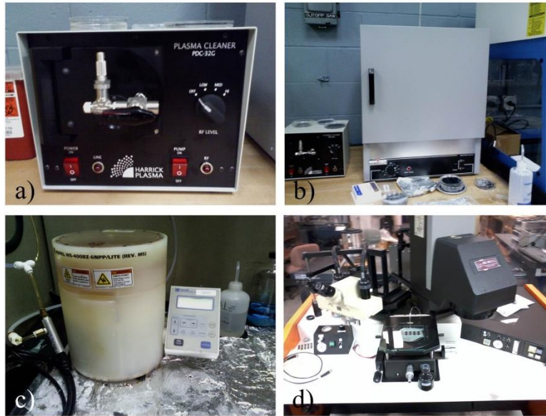
Figure 1: Images of a) plasma cleaner; b) PDMS baking oven; c) spin coater; d) mask aligner.
