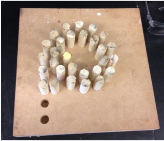
Fig. 4. The mandrels used to form the inlet scroll and cone of the scale-model hydrocyclone.
