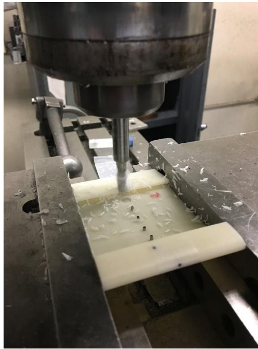
Figure 15: Utilizing a manual milling machine to remove material necessary to fit Tygon tubing
