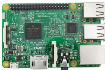
Fig. 1: Raspberry Pi 3 Model B used in the RET research
