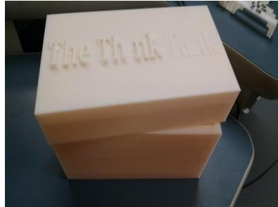
Fig. 12: First 3D print of the "Think Tank" made on the Cube Pro
